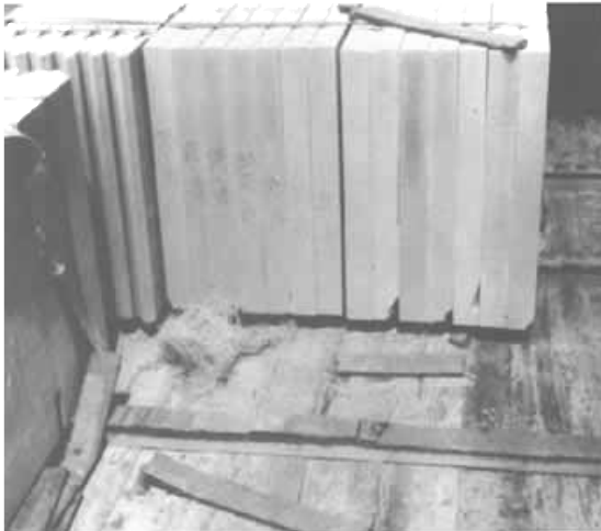
Chipped stones may be useable. Will the chips cover? Are they on the back? Can the stone be cut down, and used elsewhere?
